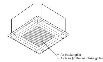
The indoor unit's intake grille can be removed for easy cleaning and maintenance.
