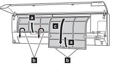
2 Remove dust by using a vacuum cleaner or by washing the filter. When you wash the filter, use neutral household detergent and warm water.
