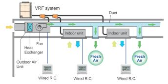
\* Make sure the connected capacity is within the range of 50% to 100% of the outdoor unit capacity. In addition, if there are mixed connections with indoor units, make the Outdoor Air Unit connection capacity 30% or less of the outdoor unit capacity.
