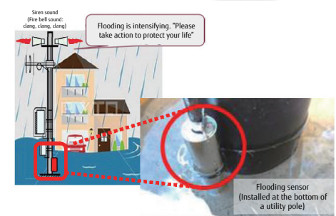
A demonstration test was conducted in Iida City, Nagano Prefecture Flooding Alert System
